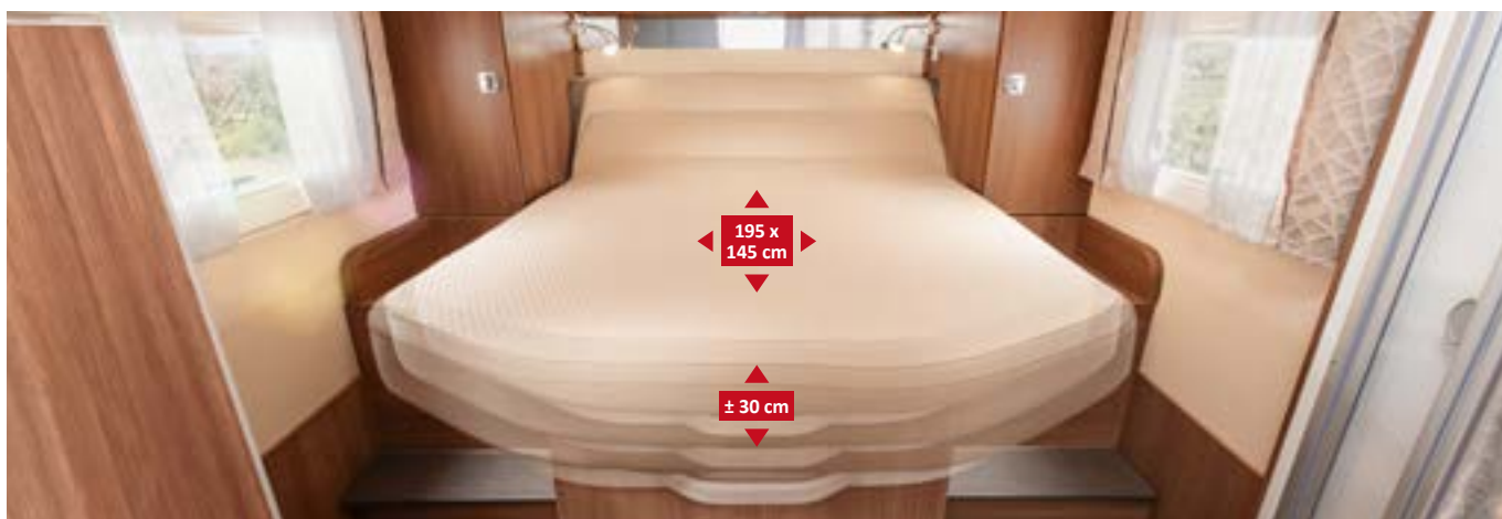
Sleeping area can be moved by 30 cm for comfortable living and sleeping configuration within a short vehicle length (T 144 QB)
