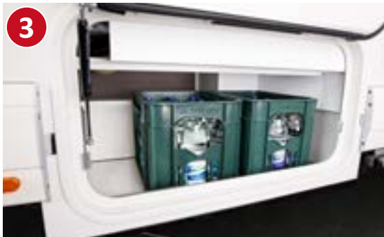
Large, additional double floor storage compartment with separate exterior hatch (driver's side)
