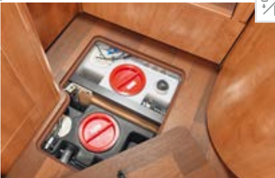
Water tanks protected from frost in heated double floor
