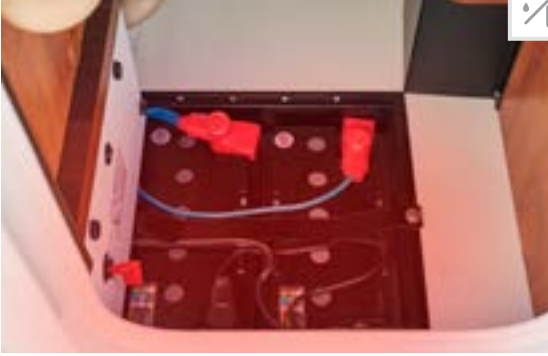
Heated battery centre with main power switch. Standard: 2 x 80 Ah gel batteries, optional 90 Ah lithium-ion battery including battery computer and separate touch display
