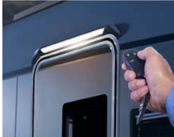
With central locking: using hand transmitter in the main key for the drivers cabin doors and activating the exterior lighting
