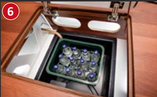
Living area floor hatch with double floor storage box (42 cm usable depth) in heated double floor
