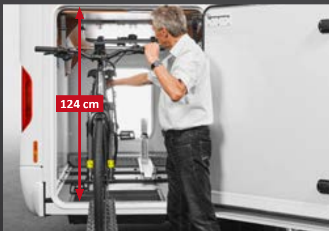
Loading height extension by simply swivelling up the interior rear bed with one hand and the additional lowered floor recess
