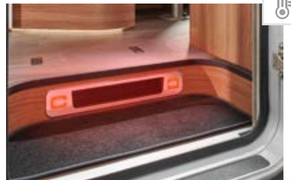
ALDE warm water central heating with numerous convectors throughout the climate storage double floor, the living area, in the scooter garage, the driver's cabin and in the cold-sensitive door entrances. Heat booster beneath the driver's seat
