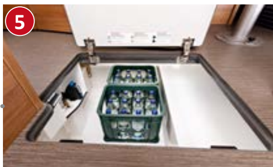
Huge living area floor hatch in the entrance area: easy to load from the outside when main cabin door is open
