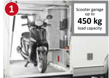
Scooter garage with additional interior height thanks to deep lowering, access from both sides via large doors at driver and passenger side
