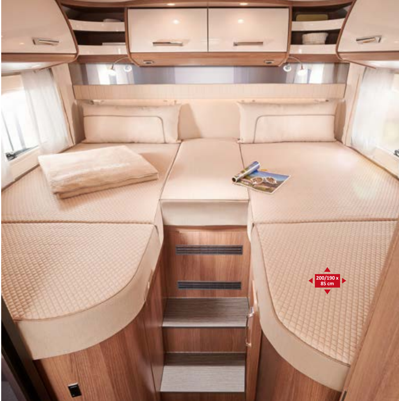
Large lengthways single beds with self-supporting head section and pull-out access steps (I 141 LE, I 143 LE, I 148 LE, I 149 LE). Convenient access to wardrobes below from front and above thanks to lift function (I 141 LE, I 143 LE, I 148 LE, 149 LE)
