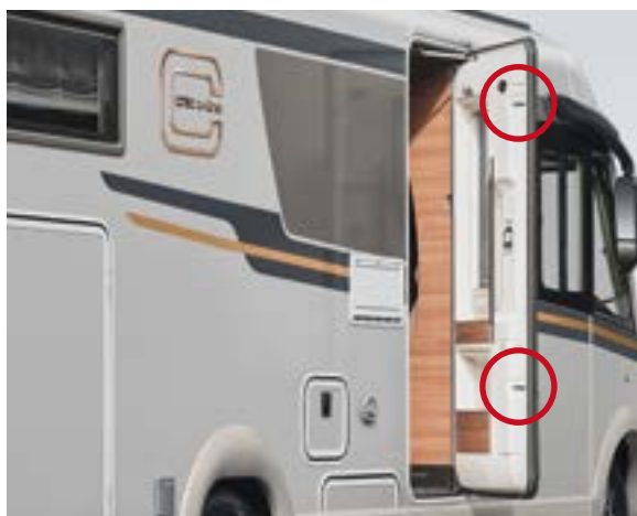
With wider passage size of 63 cm, safety double locking, extra-wide door window, pleated blackout blind and integrated insect screen roller blind
