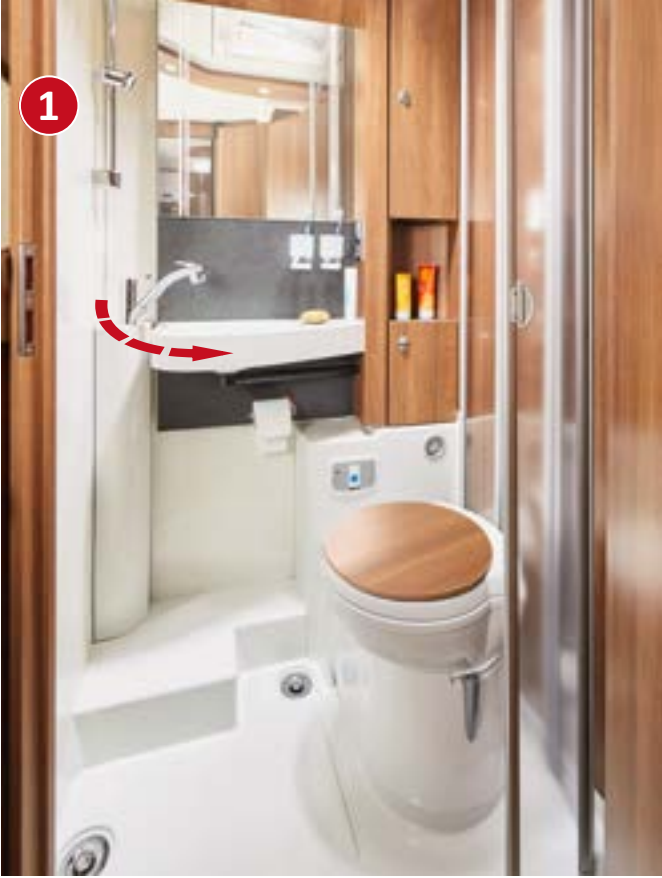
Vario swivelling washroom: washroom and toilet room 1 or shower room 2 thanks to washbasin wall mirror that can be swivelled away (I 141 LE)
