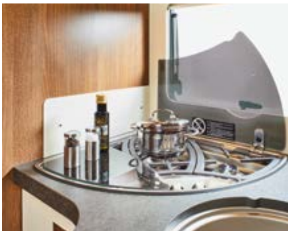
"Profi Gourmet" 3-ring hob with divided glass cover for additional storage space (I 144 LE, I 144 QB)
