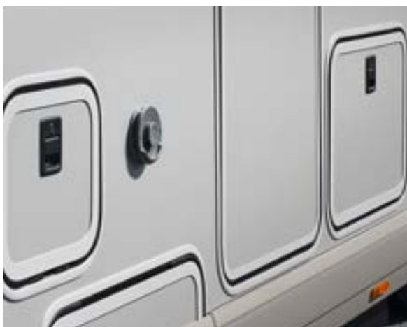
With interior hinges – integrated flat in the main body
