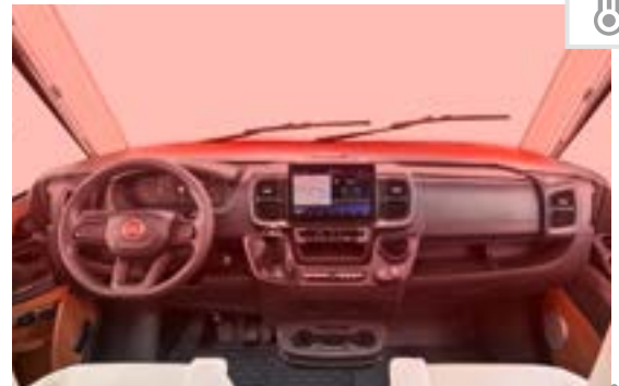
Additional heat radiation in driver's cabin area due to the heated dashboard surface, therefore less cold radiation into the driver's cabin / living area from the windscreen
