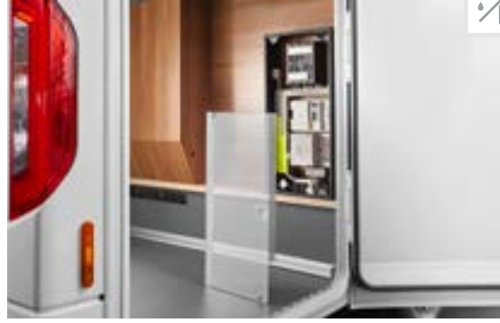
Easily accessible electrical centre in scooter garage
