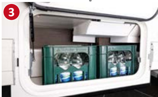
Large, additional double floor storage compartment with separate exterior hatch (at the driver's side)
