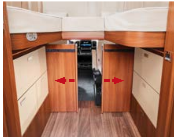
Beneath drop-down bed to prevent cold from entering from the driver's cabin in the sleeping configuration
