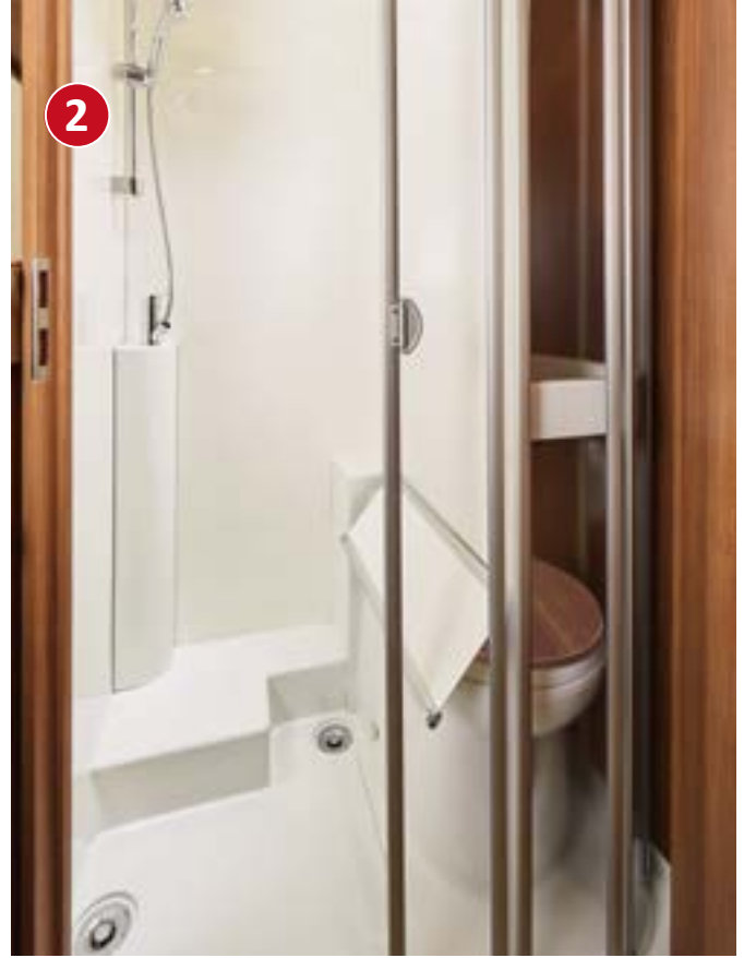
Vario swivelling washroom: washroom and toilet room 1 or shower room 2 thanks to washbasin wall mirror that can be swivelled away (I 141 LE)
