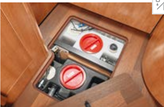
Water tanks protected from frost in heated double floor
