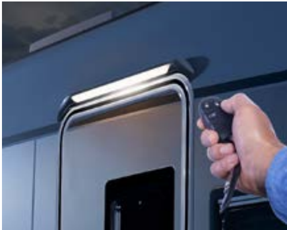
The remote control in the main key activates the central locking and the LED exterior lighting simultaneously
