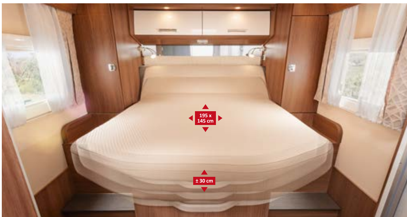
Sleeping area can be moved by 30 cm for comfortable living and sleeping conditions within a short vehicle length (I 144 LE)
