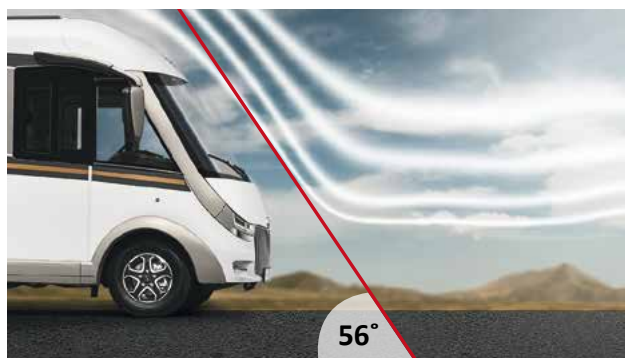
Three-dimensionally designed front with flat angle = less air resistance, lower fuel consumption and less wind noise
