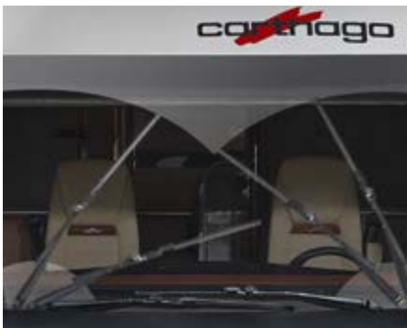
With extended wiping area and field of view (chic s-plus)
