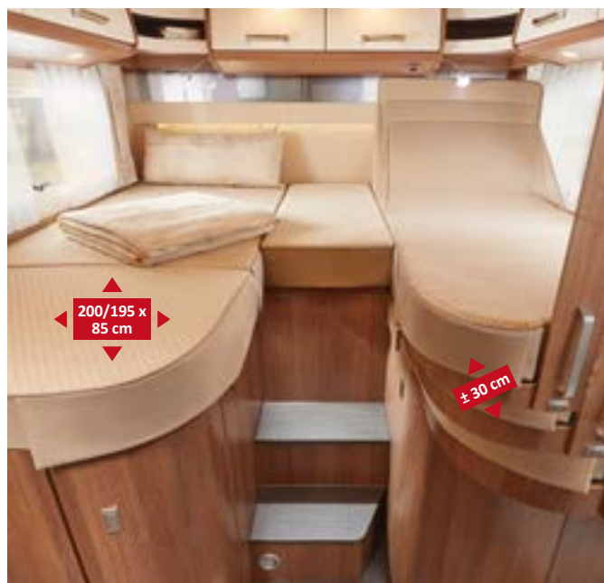
Pull-out single bed at passengers side with access steps (I 144 LE)
