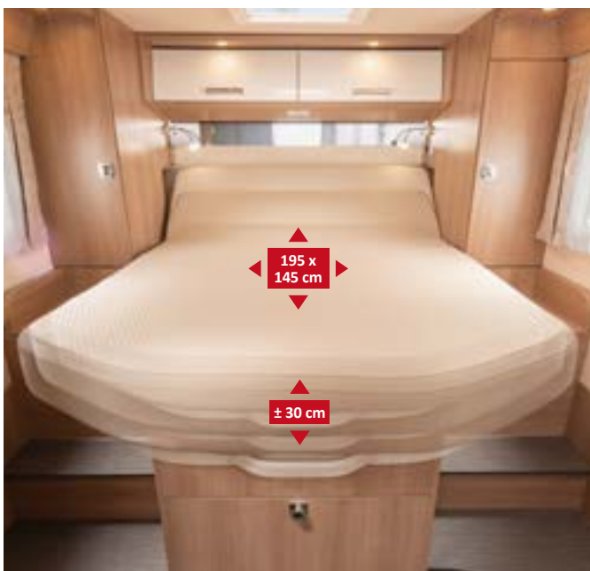
Sleeping area can be moved by 30 cm for comfortable living and sleeping conditions within a short vehicle length (I 144 LE)
