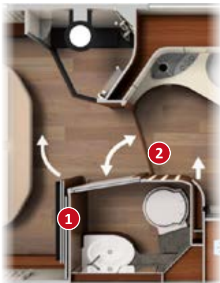
1 Pull-out TV wall and room divider for partitioning off the sleeping area. 2 Luxury washroom door with 3-way function thanks to washroom double door for partitioning off the changing room from the living area and the toilet room
