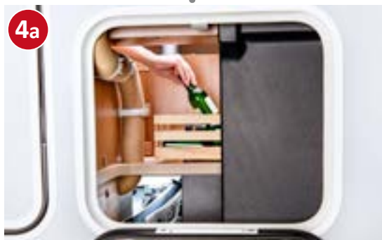
Convenient loading of the double floor storage compartment via another external hatch
