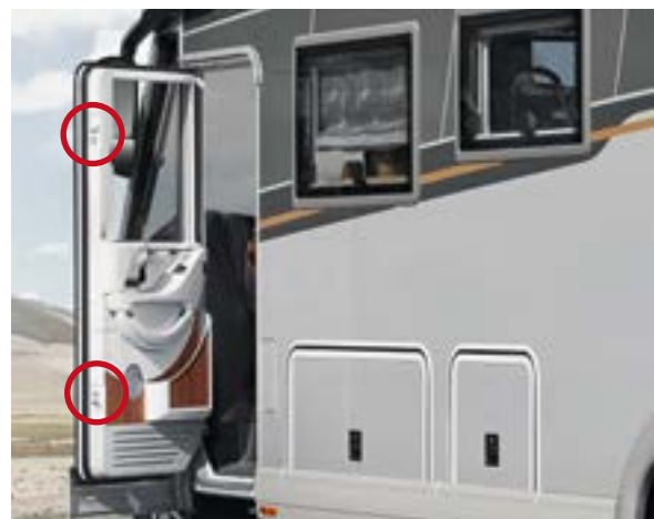
With safety double locking system, electric window and low door entrance
