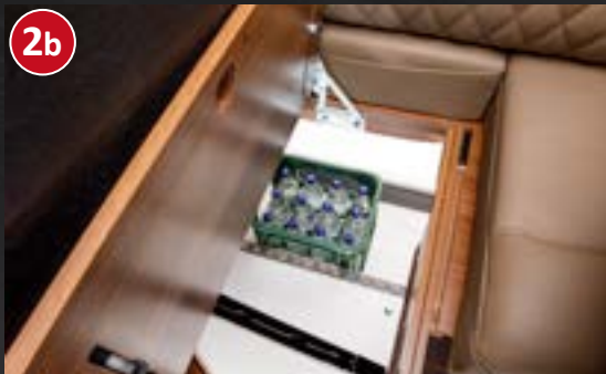
Easy removal of storage compartment contents from the inside via the fold-up seat bench cover of the L-shaped lounge seating area
